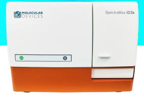
The streamlined SpectraMax® iD3s tunable monochromator-based microplate reader with temperature control provides an affordable solution for measuring absorbance, fluorescence, and luminescence. The reader's optional upgrades include dual injection and support for live cell assays with environmental controls  $(CO_2/O_2)$  and advanced shaking.
