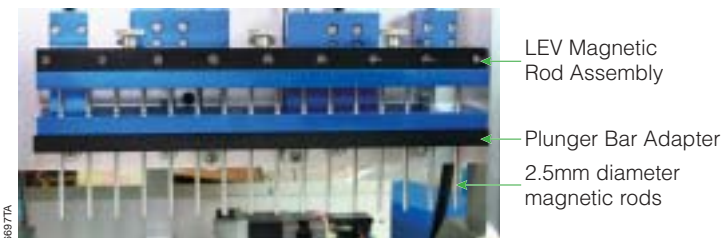
Figure 2. Maxwell® 16 Instrument hardware set to LEV configuration. Refer to the Maxwell® 16 Instrument Technical Manual #TM274 to reconfigure your instrument to the LEV hardware configuration.
